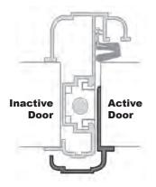
Add the Astragal **Security**Strip to any outswing double door combination for added security and clean finished appearance eliminating the reveal between the doors
